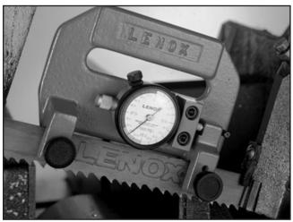
Figure 51. H5408 Blade Tensioning Gauge.
